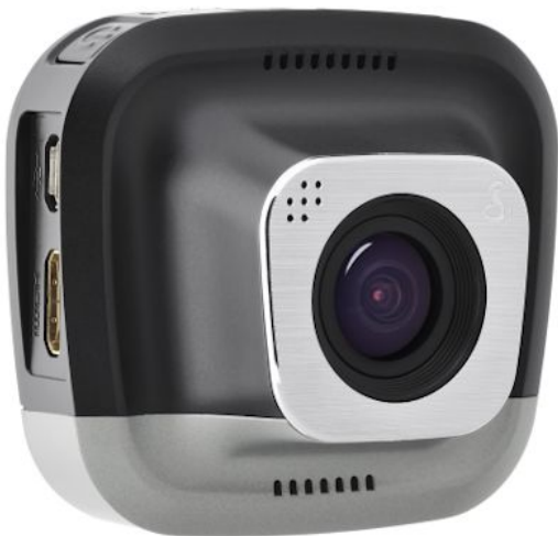
Figure 5. Cobra's Drive HD Dash Cam not only records the action ahead, it connects to smartphones with Bluetooth for GPS iRadars data. Source: Cobra
