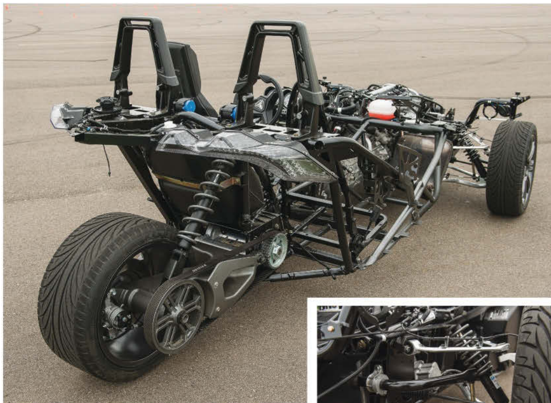
WILD MACHINE: Big front anti-roll bar, right, keeps rear tire flush with ground.
