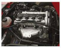
Power comes from a proven 173 hp, 2.4-liter Ecotec four-banger sourced from General Motors.
